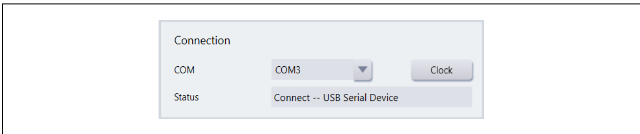
Figure 2-21 Status displayed in Connection screen when connection is established
