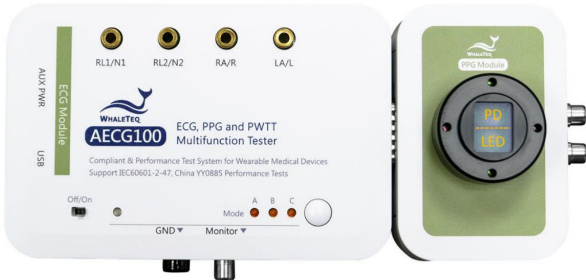
Figure 2. WhaleTeq AECG100 Tester with PPG Module Attached
