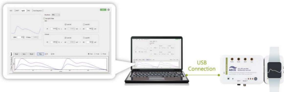
Figure 1. SP02 Test Setup with WhaleTeq AECG100
