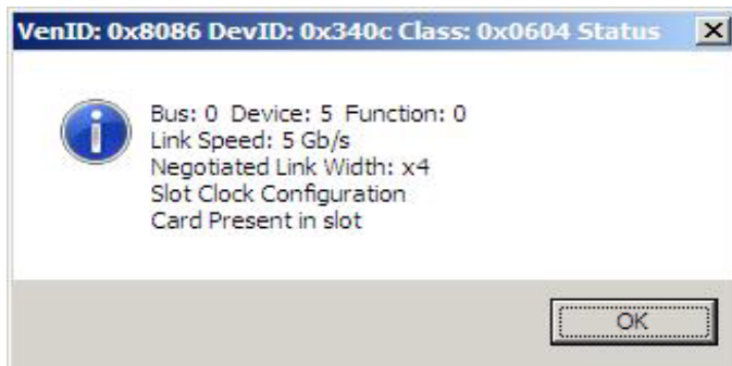
Figure 3 Status of a PCI Express Device Not Manufactured by IDT
