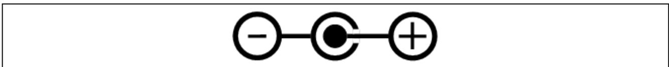
**Figure 10.2 Pin Assignments of the Power-Supply Connector**
