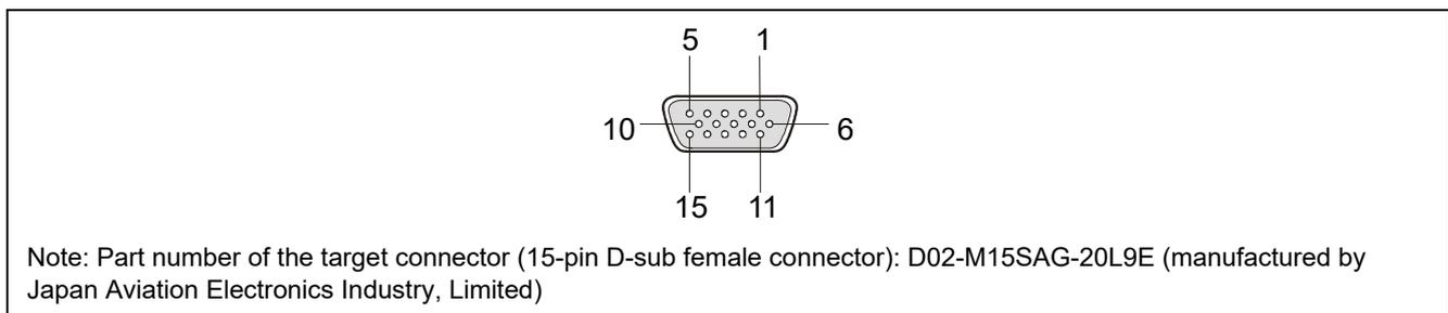
**Figure 10.9 Pin Assignments of the Target Connector (15-Pin D-Sub Female Connector)**
