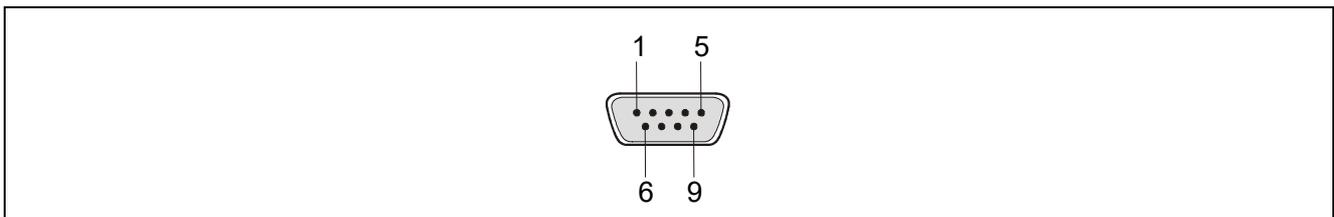
**Figure 10.4 Pin Assignments of the Serial Connector**
