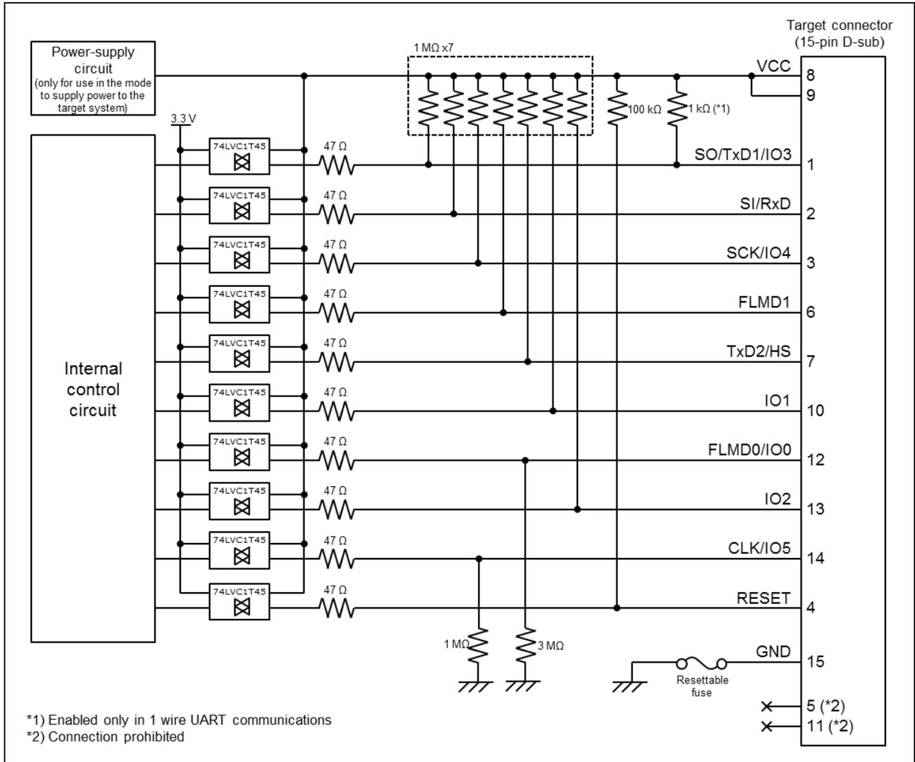
Figure C.1 Equivalent Circuits of the Target Interface
