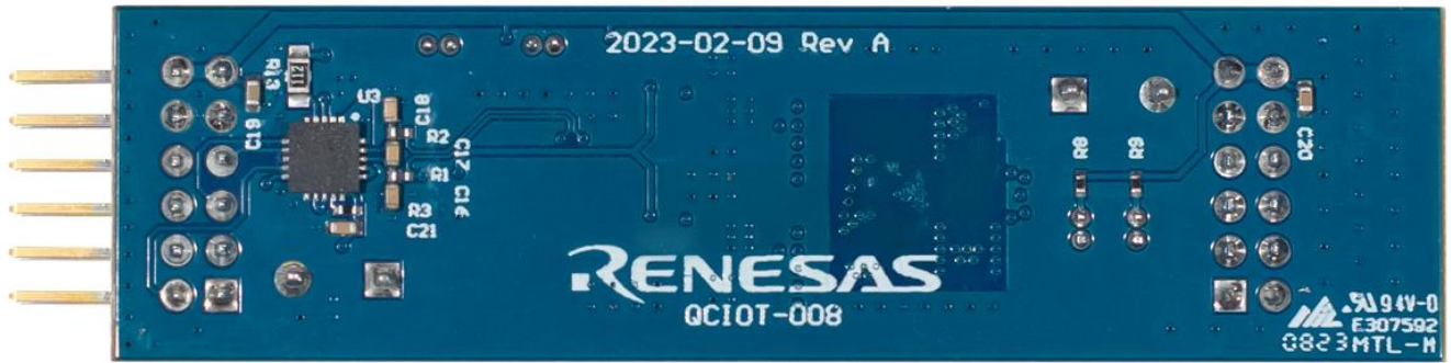
Figure 5. QCIOT-COMPPOCZ Evaluation Board (Bottom)
