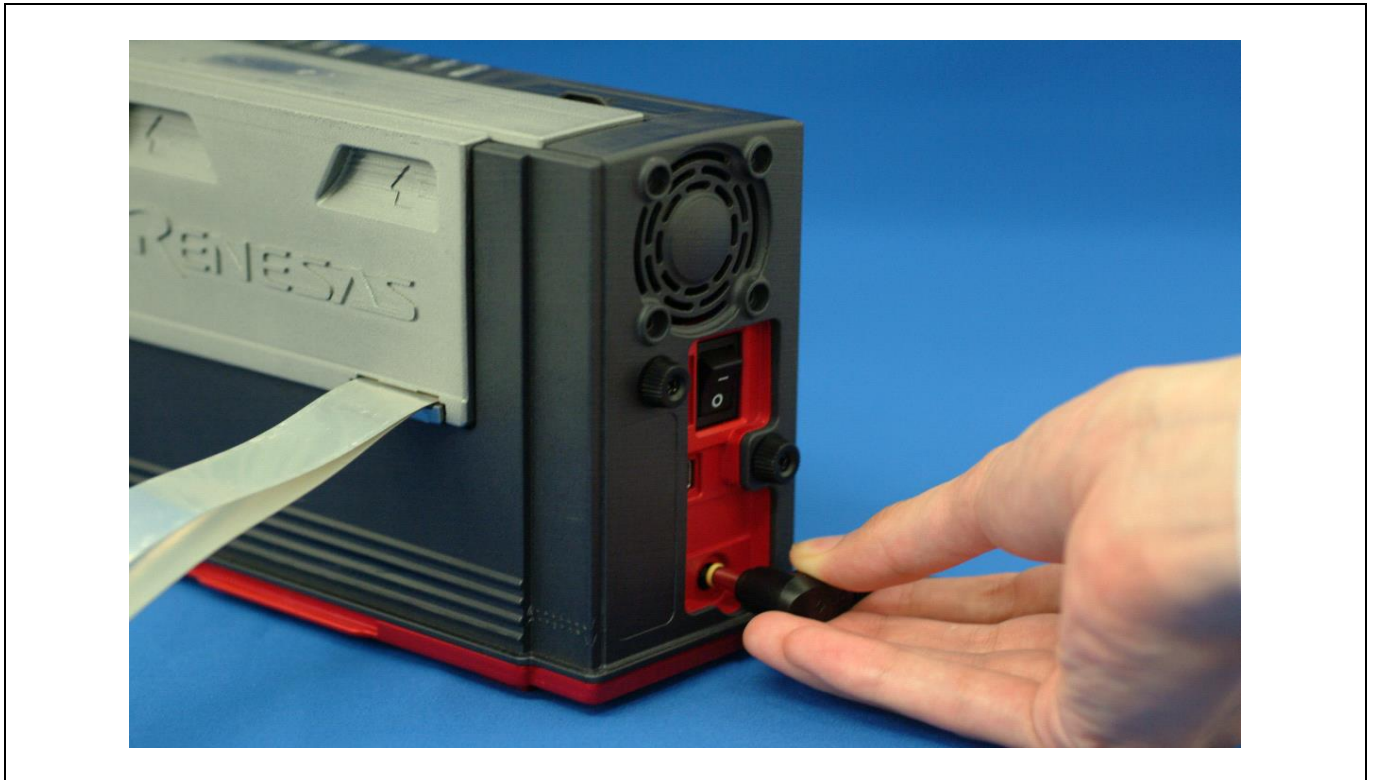
Figure 2.5 Connecting the emulator power supply
