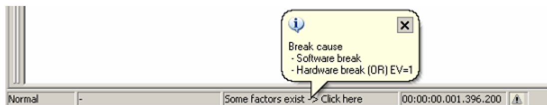
Figure 5.15 Checking the source of a break
