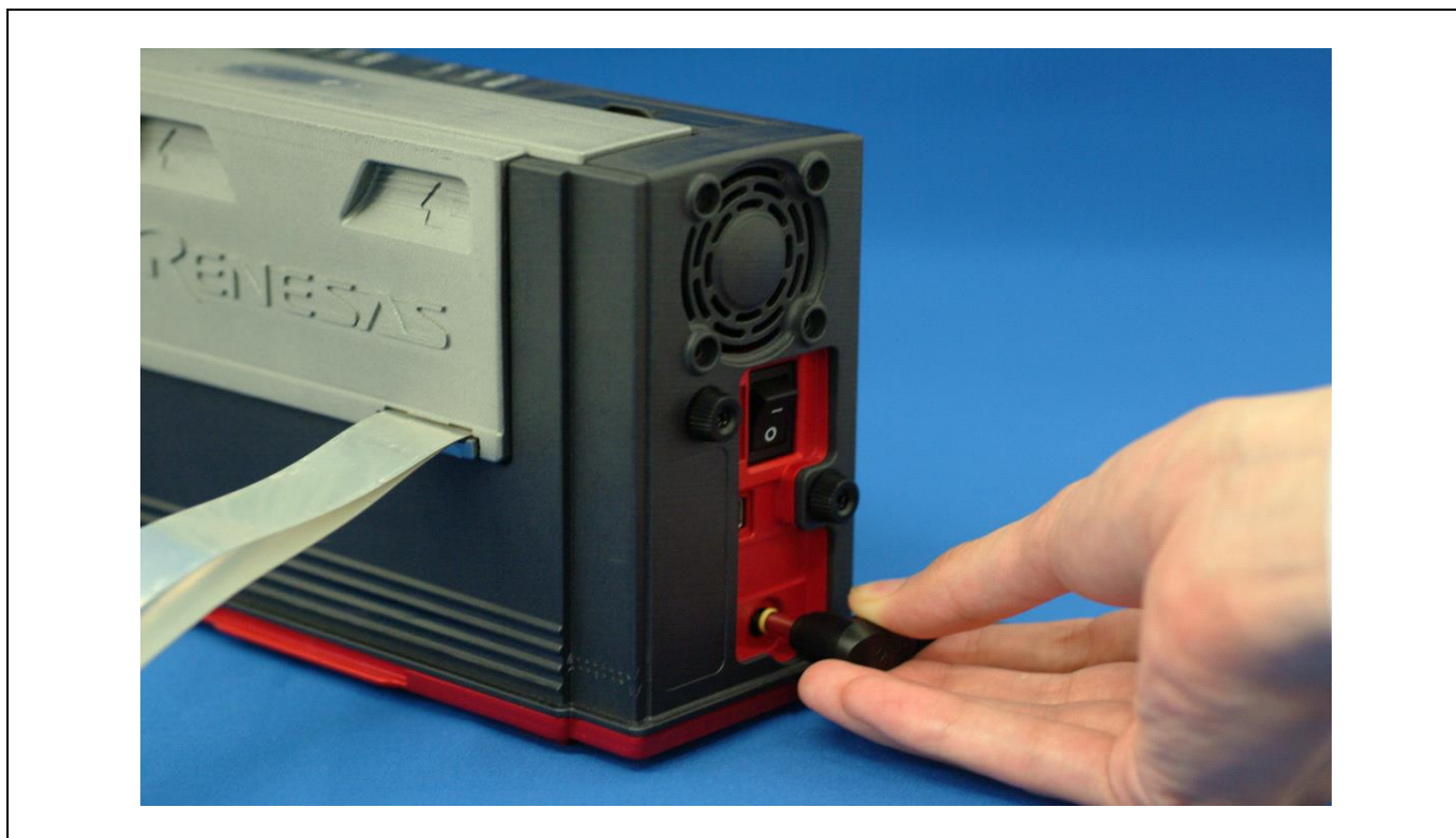
Figure 2.5 Connecting the emulator power supply
