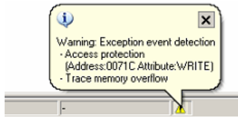
Figure 5.19 Example of Warning Display when Exceptional Events Occur
