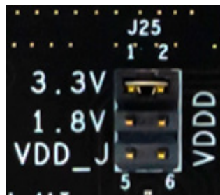
Figure 3. Power Source Selector for VDDD
