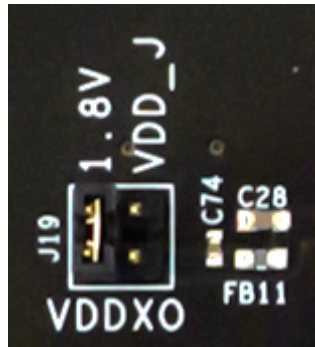
Figure 2. Power Source Selector Example
