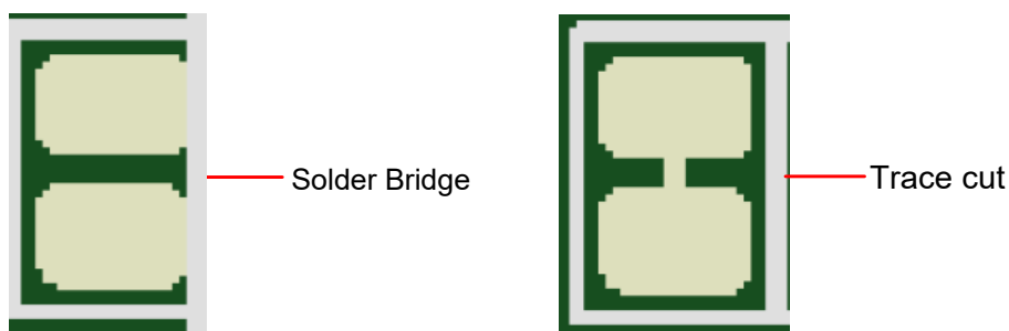
Figure 6-1 Solder Bridge and Trace Cut
