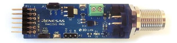
Figure 1. RH4Z2501-PMOD (Default Jumper Setting)
