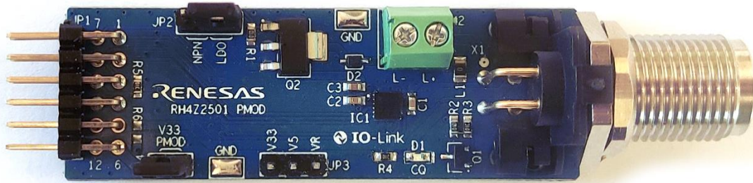
Figure 1. RH4Z2501-PMOD (Default Jumper Setting)
