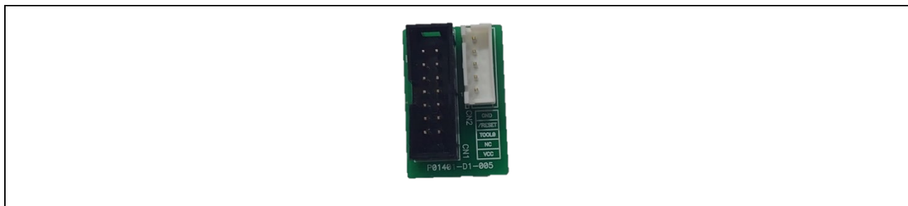
Figure 8-7 Conversion Boards (P014012-1-005)
