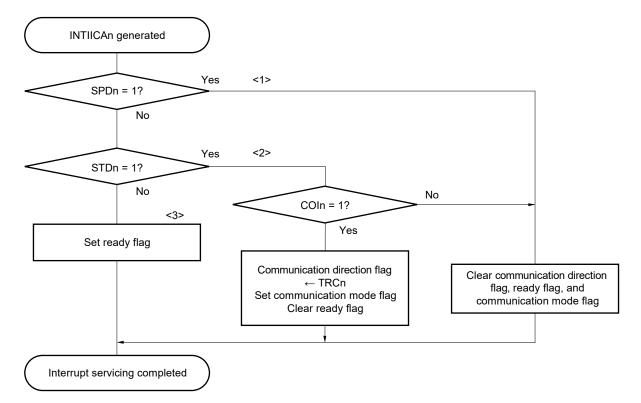
Figure 15-31. Slave Operation Flowchart (2)
