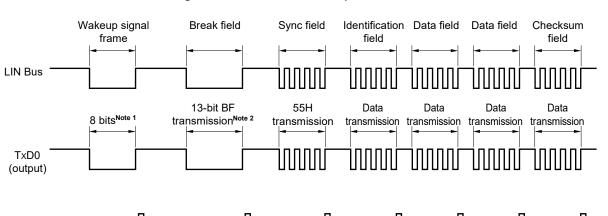
Figure 14-98. Transmission Operation of LIN
