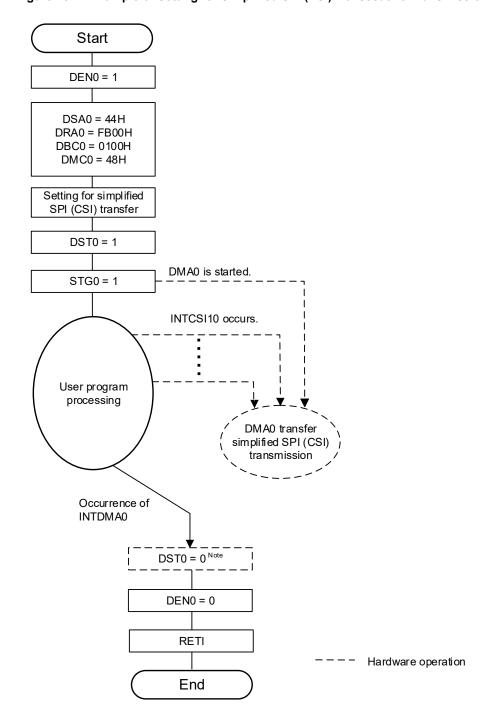
Figure 18-7. Example of Setting for Simplified SPI (CSI) Consecutive Transmission
