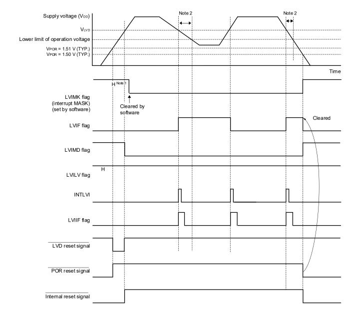
Figure 24-6. Timing of Voltage Detector Internal Interrupt Signal Generation (Option Byte LVIMDS1, LVIMDS0 = 0, 1)
