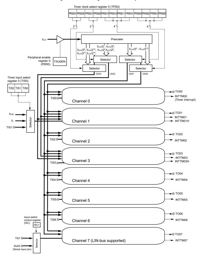
Figure 6-1. Entire Configuration of Timer Array Unit
