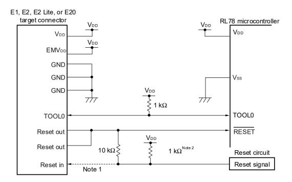
Notes 1. The connection shown as a broken line is not required for serial programming.
