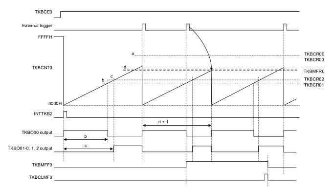
Figure 7-64. Maximum Frequency Limit Function
