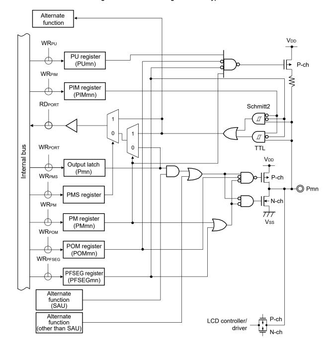
Figure 2-15. Pin Block Diagram for Pin Type 8-5-10
