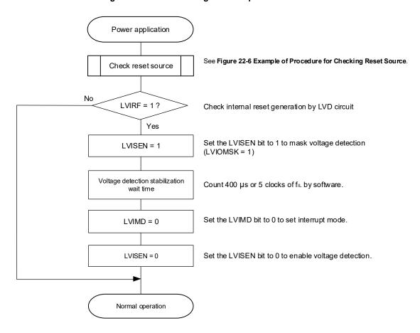
Figure 24-9. Initial Setting of Interrupt and Reset Mode
