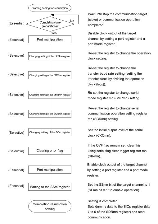
Figure 14-36. Procedure for Resuming Master Reception
