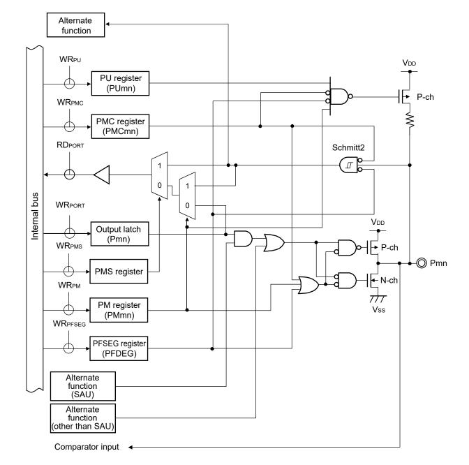
Figure 2-12. Pin Block Diagram for Pin Type 7-6-9
