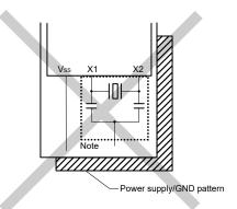
Note Do not place a power supply/GND pattern under the wiring section (section indicated by a broken line in the figure) of the X1 and X2 pins and the resonators in a multi-layer board or double-sided board.
