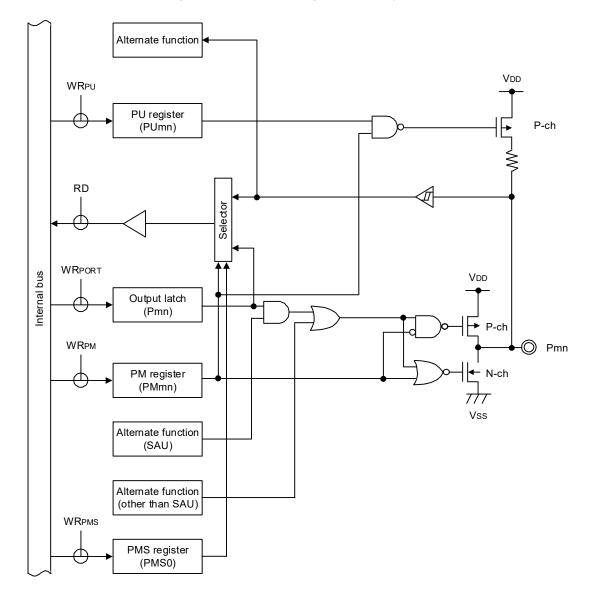
Figure 2-5. Pin Block Diagram for Pin Type 7-1-3
