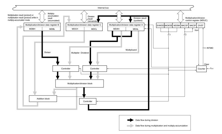
Figure 17-1. Block Diagram of Multiplier and Divider/Multiply-Accumulator
