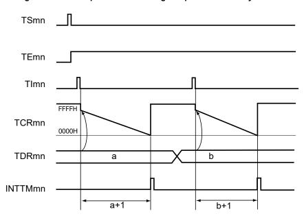
Figure 6-60. Example of Basic Timing of Operation as Delay Counter
