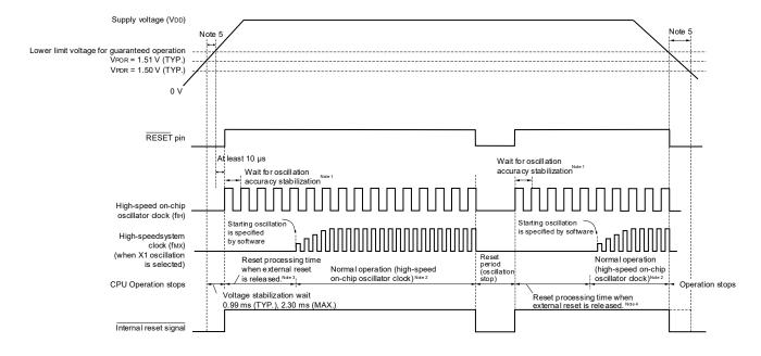
Notes 1. The internal reset processing time includes the oscillation accuracy stabilization time of the high-speed onchip oscillator clock.
