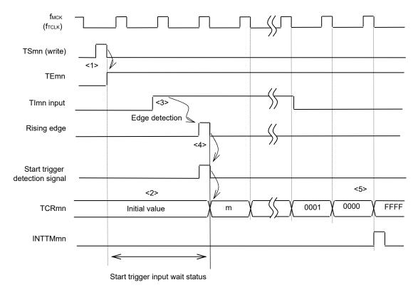
Figure 6-30. Operation Timing (In One-count Mode)
