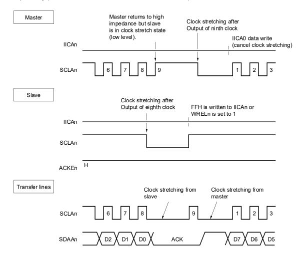
Figure 15-20. Clock stretching (2/2)
