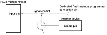
In the flash memory programming mode, a signal output by another device will conflict with the signal output by the dedicated flash memory programmer. Therefore, isolate the signal of another device.
