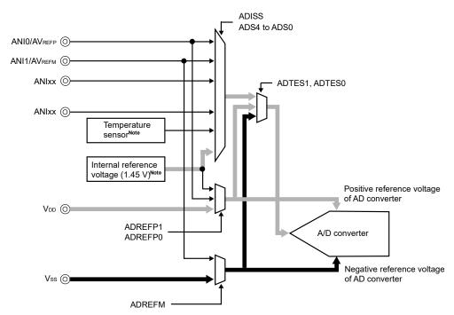
Figure 25-15. Configuration of A/D Test Function
