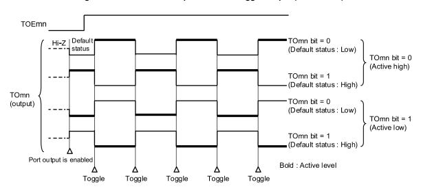
Figure 6-34. TOmn Pin Output Status at Toggle Output (TOMmn = 0)
