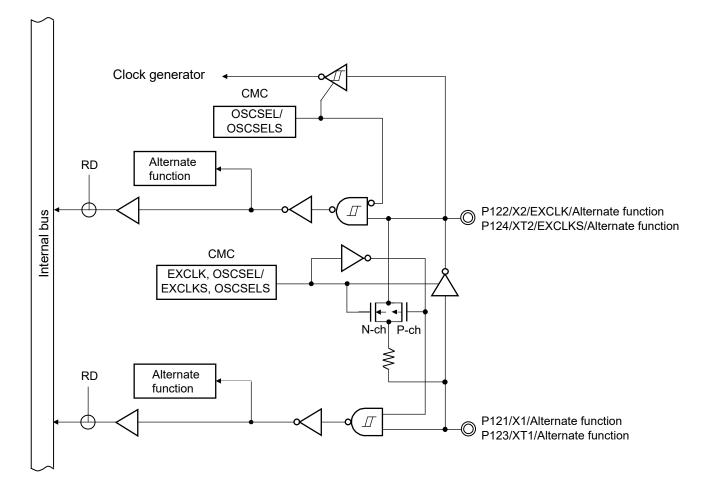
Figure 2-3. Pin Block Diagram for Pin Type 2-2-1
