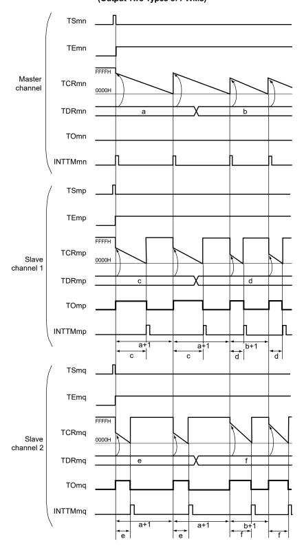
Figure 6-74. Example of Basic Timing of Operation as Multiple PWM Output Function (Output Two Types of PWMs)
