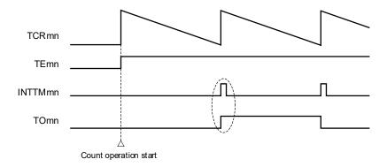
When MDmn0 is set to 1, a timer interrupt (INTTMmn) is output at count operation start, and TOmn performs a toggle operation.
