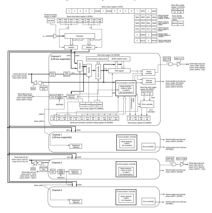
Figure 14-1. Block Diagram of Serial Array Unit 0
