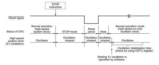
Note For the reset processing time, see CHAPTER 22 RESET FUNCTION. For the reset processing time of the power-on-reset circuit (POR) and voltage detector (LVD), see CHAPTER 23 POWER-ON-RESET CIRCUIT.
