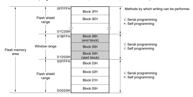
Figure 28-11. Flash Shield Window Setting Example (Target Devices: R5F10WLE, Start Block: 04H, End Block: 06H)
