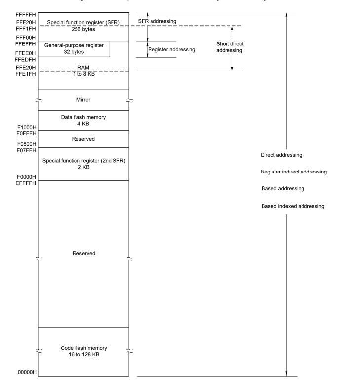
Figure 3-8. Correspondence Between Data Memory and Addressing
