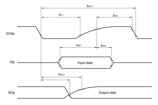
Simplified SPI (CSI) mode serial transfer timing (master mode) (during communication at different potential) (When DAPmn = 0 and CKPmn = 1, or DAPmn = 1 and CKPmn = 0.)
