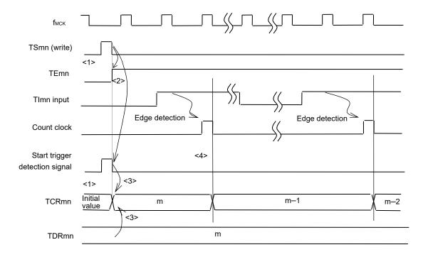
Figure 6-28. Operation Timing (In Event Counter Mode)
