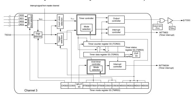
Figure 6-4. Internal Block Diagram of Channels 3 of Timer Array Unit
