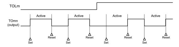
Remarks 1. Set: The output signal of the TOmn pin changes from inactive level to active level.
