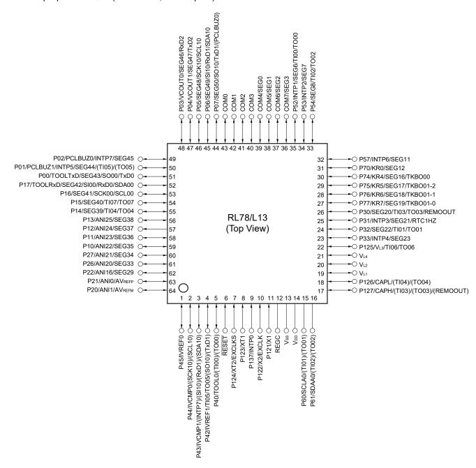
Caution Connect the REGC pin to Vss via a capacitor (0.47 to 1  $\mu$ F).
