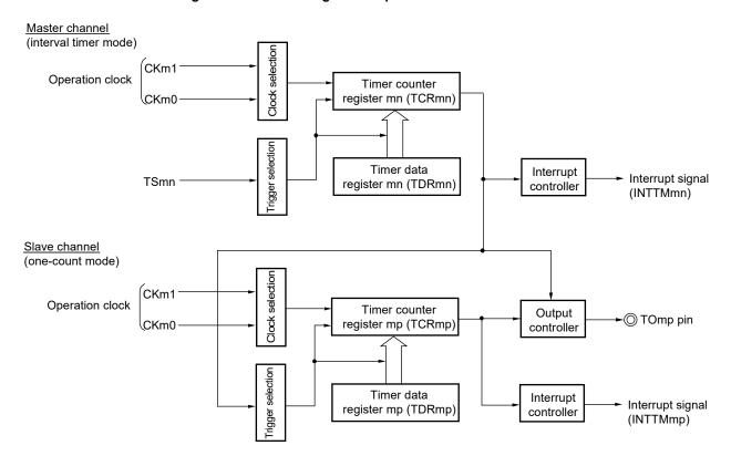
Figure 6-68. Block Diagram of Operation as PWM Function
