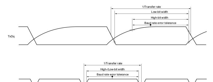
**Remarks 1.** R<sub>b</sub>[Ω]: Communication line (TxDq) pull-up resistance, C<sub>b</sub>[F]: Communication line (TxDq) load capacitance, V<sub>b</sub>[V]: Communication line voltage
