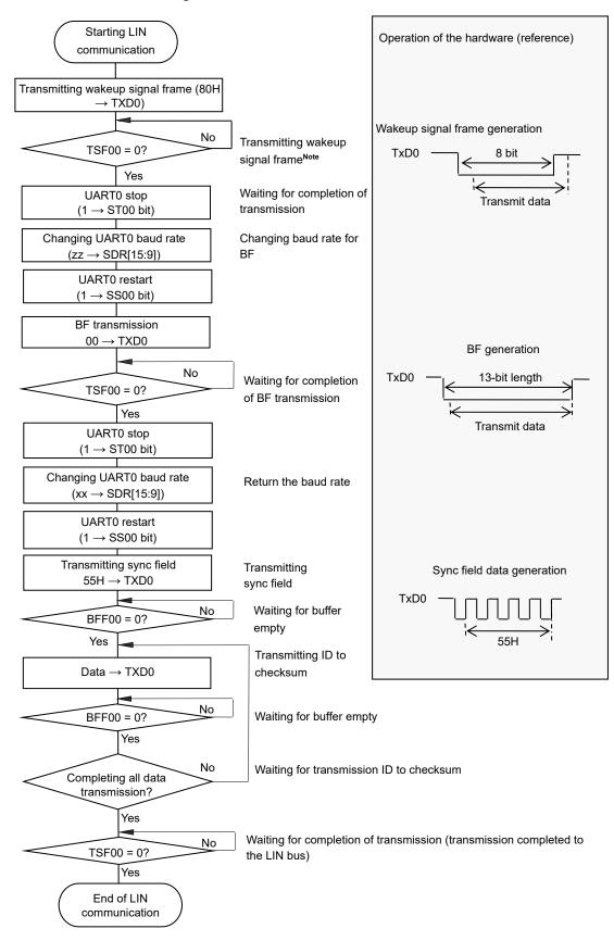
Figure 14-99. Flowchart for LIN Transmission
