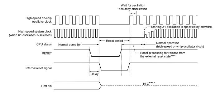
Figure 22-2. Timing of Reset by RESET Input
