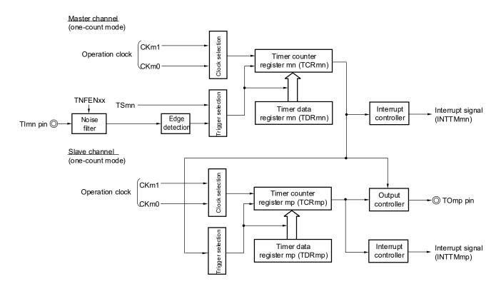
Figure 6-63. Block Diagram of Operation as One-Shot Pulse Output Function
