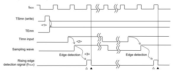
Figure 6-26. Timing of fclκ and count clock (fτclκ) (When CCSmn = 1, noise filter unused)
