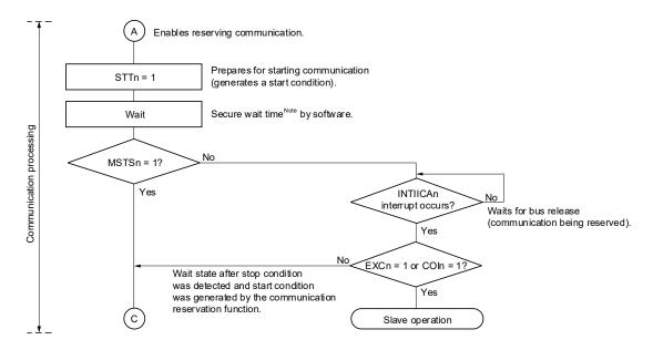
Figure 15-29. Master Operation in Multi-Master System (2/3)
