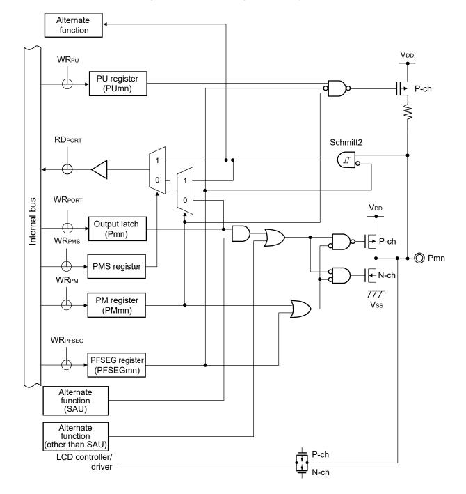
Figure 2-6. Pin Block Diagram for Pin Type 7-5-4
