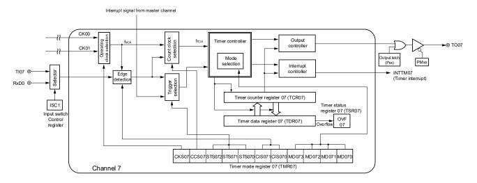
Figure 6-6. Internal Block Diagram of Channels 7 of Timer Array Unit
