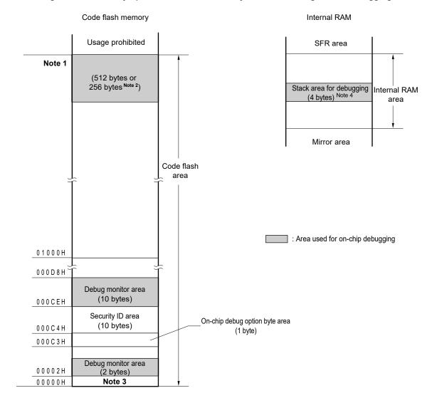
Figure 29-2. Memory Spaces Allocated for Use by the Monitor Program for Debugging
