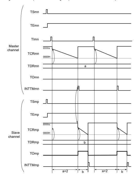
Figure 6-64. Example of Basic Timing of Operation as One-Shot Pulse Output Function
