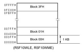
Correspondence between the address values and block numbers in the flash memory are shown below.
