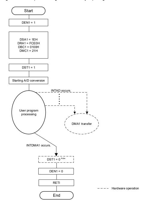
Figure 18-8. Example of Setting of Consecutively Capturing A/D Conversion Results
