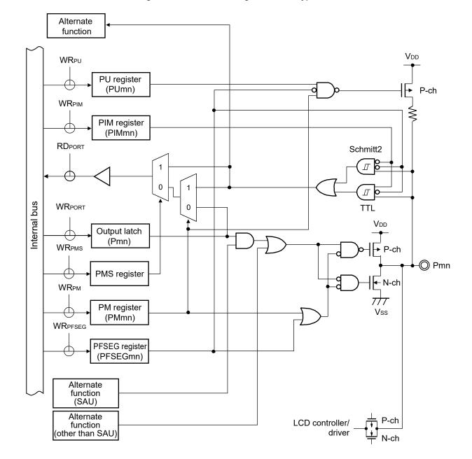
Figure 2-14. Pin Block Diagram for Pin Type 8-5-4
