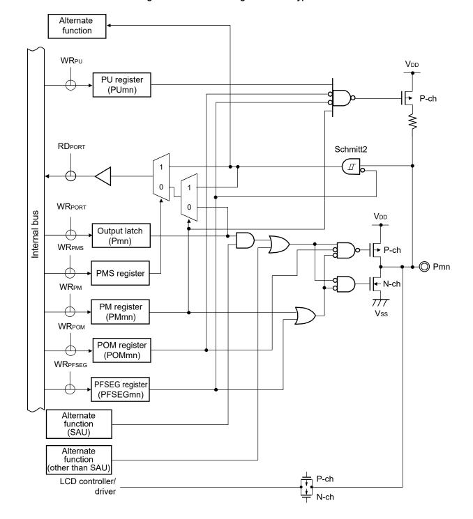
Figure 2-9. Pin Block Diagram for Pin Type 7-5-10
