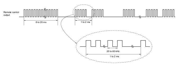
Figure 6-78. Remote Control Output
