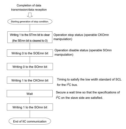
Figure 14-114. Flowchart of Stop Condition Generation
