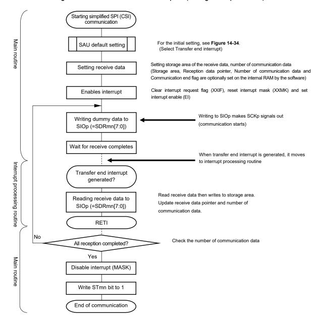
Figure 14-38. Flowchart of Master Reception (in Single-Reception Mode)
