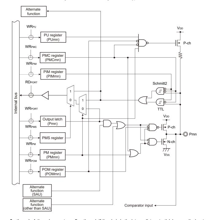
Figure 2-16. Pin Block Diagram for Pin Type 8-6-4
