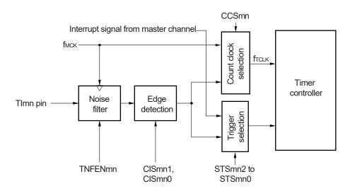
Figure 6-41. Input Circuit Configuration
