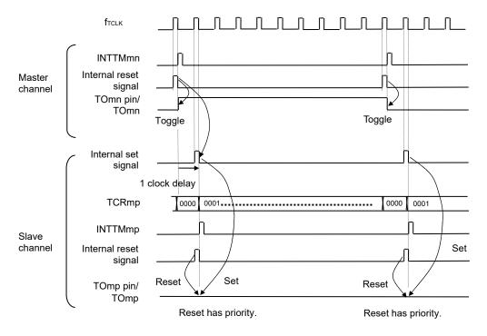
**Remarks 1.** Internal reset signal: TOmn pin reset/toggle signal Internal set signal: TOmn pin set signal
