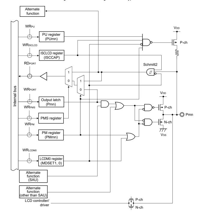
Figure 2-7. Pin Block Diagram for Pin Type 7-5-5
