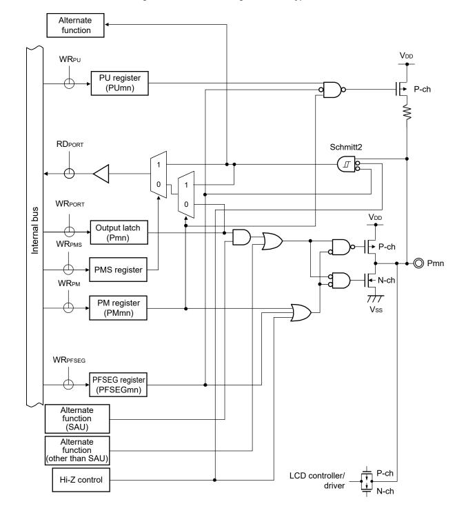
Figure 2-10. Pin Block Diagram for Pin Type 7-5-16
