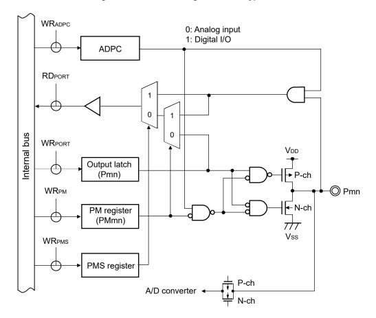
Figure 2-4. Pin Block Diagram for Pin Type 4-3-3
