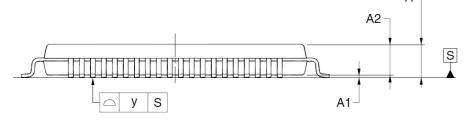
**NOTE**Each lead centerline is located within 0.08 mm of its true position at maximum material condition.
