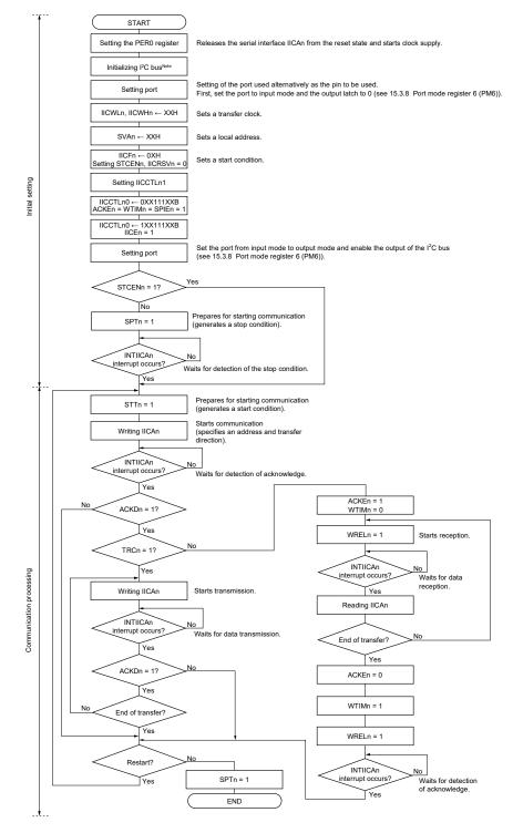
Figure 15-28. Master Operation in Single-Master System
