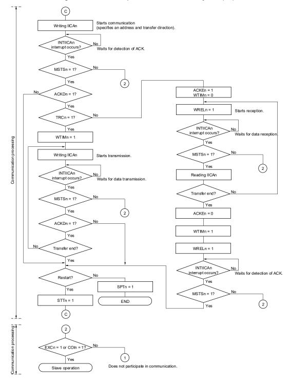
Figure 15-29. Master Operation in Multi-Master System (3/3)
