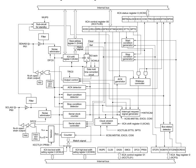
Figure 15-1. Block Diagram of Serial Interface IICA0
