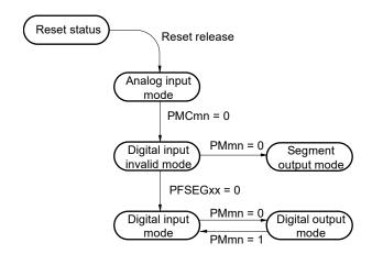
Caution Be sure to set the segment output mode before segment output starts (while SCOC of LCD mode register 1 (LCDM1) is 0).
