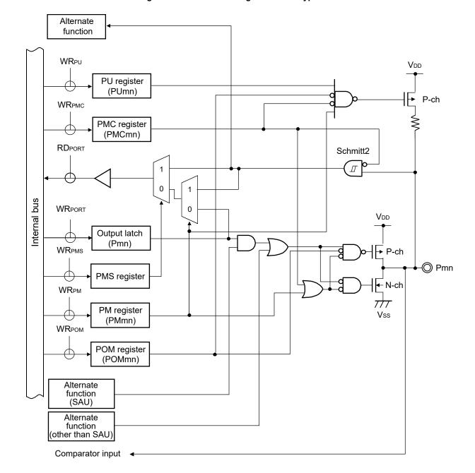
Figure 2-11. Pin Block Diagram for Pin Type 7-6-4
