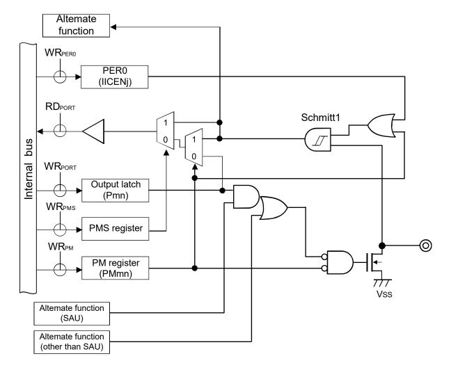
Figure 2-17. Pin Block Diagram for Pin Type 12-1-3
