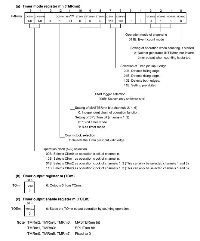
Figure 6-49. Example of Set Contents of Registers in External Event Counter Mode (1/2)
