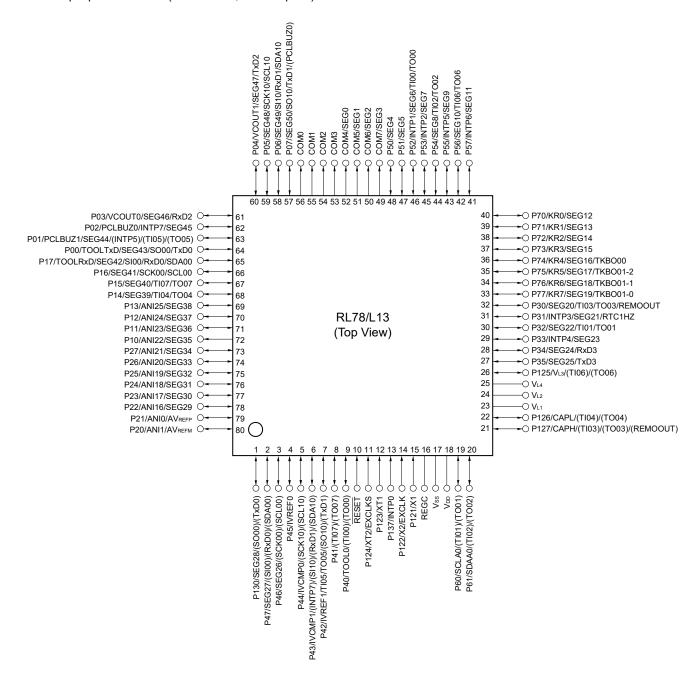
Caution Connect the REGC pin to Vss via a capacitor (0.47 to 1 µF).
