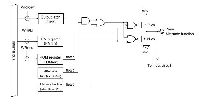
Figure 4-11. Basic Configuration of Output Circuit for Pins
