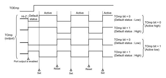
Figure 6-35. TOmp Pin Output Status at PWM Output (TOMmp = 1)
