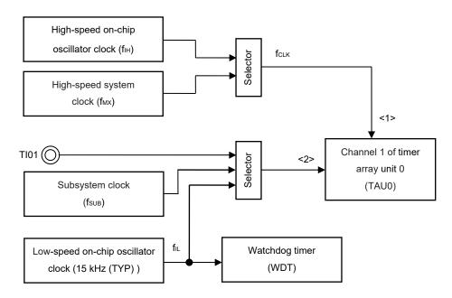
If input pulse interval measurement results in an abnormal value, it can be concluded that the clock frequency is abnormal.
