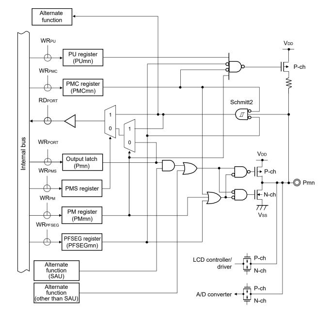
Figure 2-13. Pin Block Diagram for Pin Type 7-10-3
