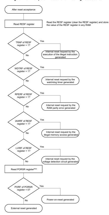
Figure 22-6. Example of Procedure for Checking Reset Source
