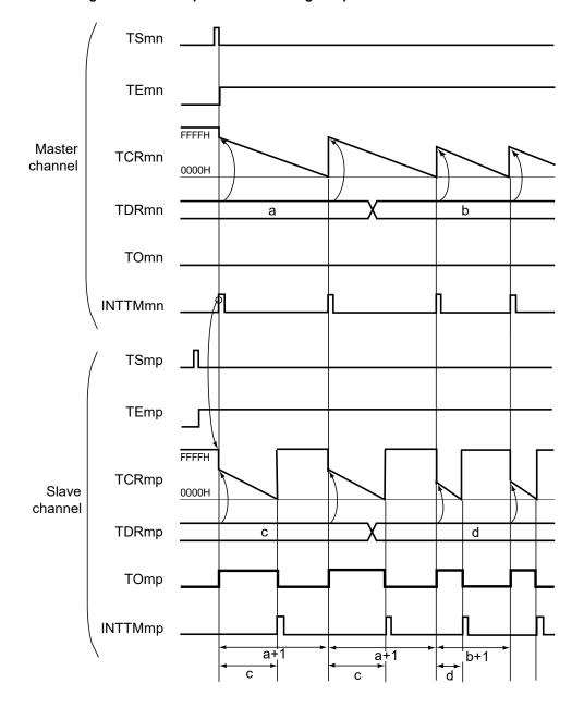
Figure 6-69. Example of Basic Timing of Operation as PWM Function
