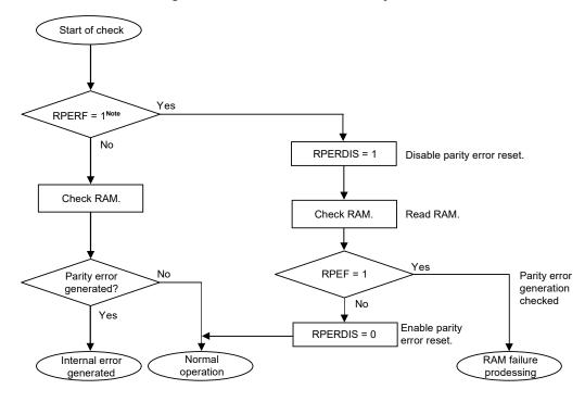
Figure 25-8. Flowchart of RAM Parity Check
