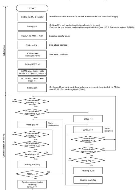
Figure 15-30. Slave Operation Flowchart (1)
