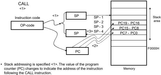
The values of PC bits 19 to 16, 15 to 8, and 7 to 0 are stored in addresses SP - 1, SP - 2, SP - 3, and SP - 4, respectively <2>.
