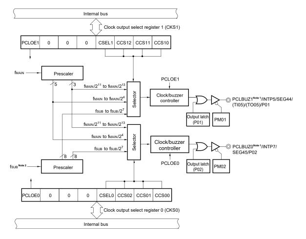
Figure 10-1. Block Diagram of Clock Output/Buzzer Output Controller
