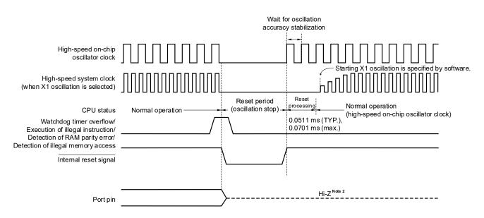
Figure 22-3. Timing of Reset Due to Watchdog Timer Overflow, Execution of Illegal Instruction,
