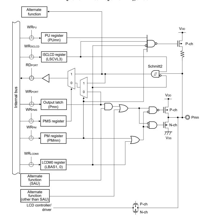
Figure 2-8. Pin Block Diagram for Pin Type 7-5-6
