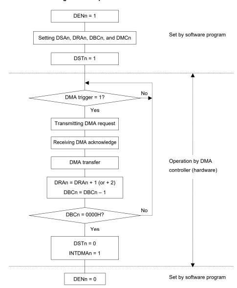
Figure 18-6. Operation Procedure
