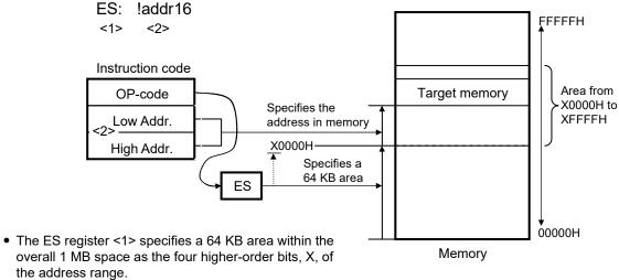
A 16-bit address <2> in the area from X0000H to XFFFFH and the ES register <1> specify the target location; this is used for access to fixed data other than that in mirrored areas.
