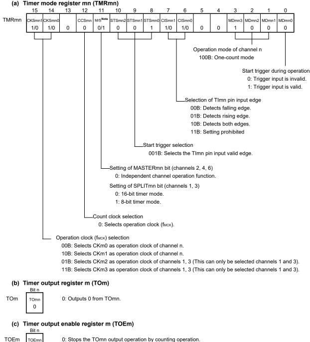
Figure 6-61. Example of Set Contents of Registers to Delay Counter (1/2)
