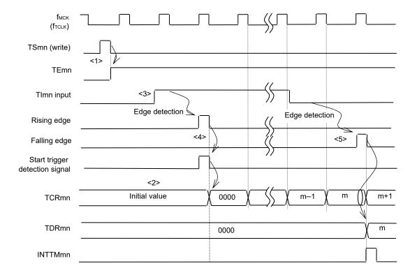
**Remark** The above figure indicates the timing when the noise filter is not used. When the noise filter is turned on, edge detection is delayed by 2 fmcκ cycles (it sums up to 3 to 4 cycles) from Tlmn input. The error per one cycle occurs because the Tlmn input is not synchronous with the count clock (fmcκ).
