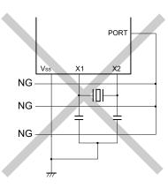
(c) The X1 and X2 signal line wires cross.
