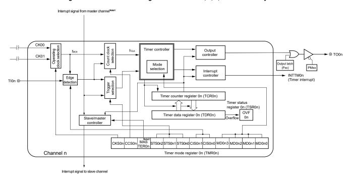
Figure 6-2. Internal Block Diagram of Channels 0, 2, 4, 6 of Timer Array Unit
