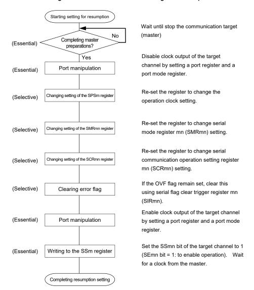
Figure 14-60. Procedure for Resuming Slave Reception
