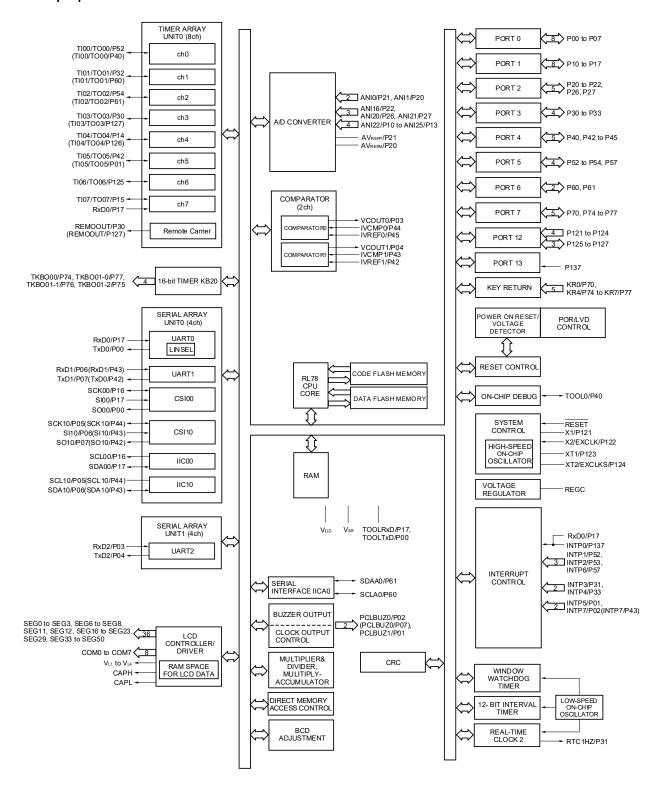
**Remark** Functions in parentheses in the above figure can be assigned via settings in the peripheral I/O redirection register (PIOR). See **Figure 4-8 Format of Peripheral I/O Redirection Register (PIOR)**.
