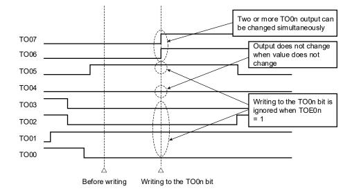
Figure 6-39. TO0n Pin Statuses by Collective Manipulation of TO0n Bit
