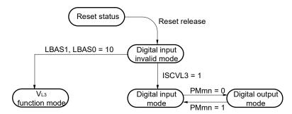
Caution Be sure to set the  $V_{L3}$  function mode before segment output starts (while SCOC of LCD mode register 1 (LCDM1) is 0).
