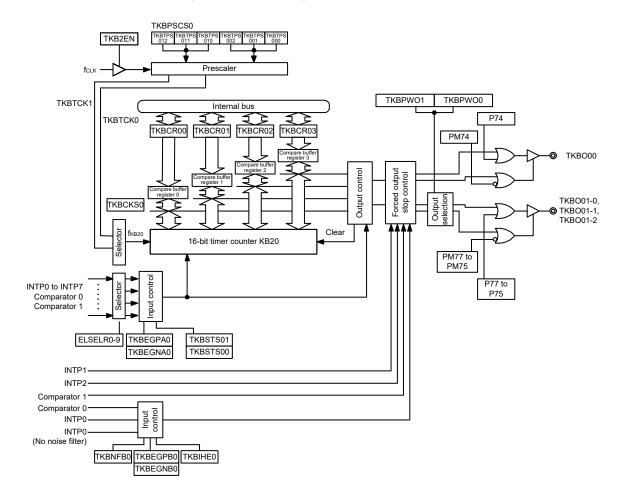
Figure 7-1. Block Diagram of 16-bit Timer KB20
