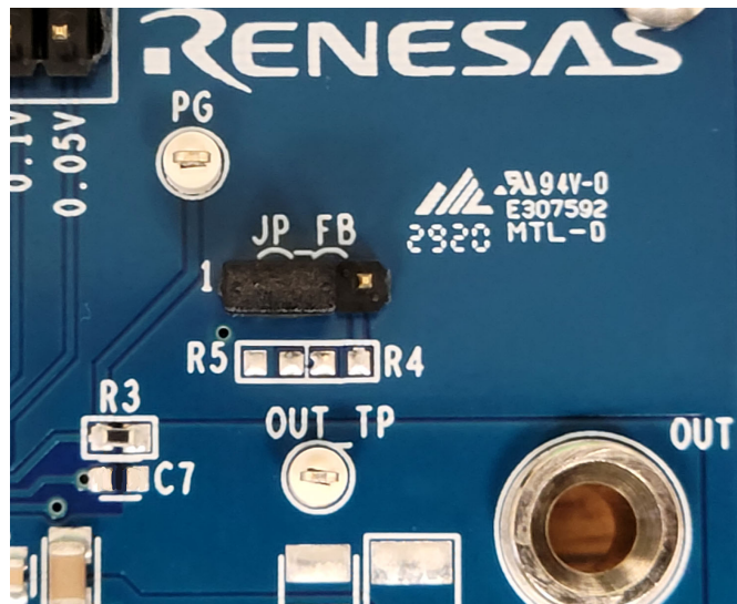
Figure 2. RTKA214023DE0010BU JP_FB Jumper for Voltage Set Pin Configuration
