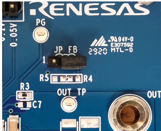
Figure 4. RTKA214023DE0000BU JP_FB Jumper for External Feedback Configuration
