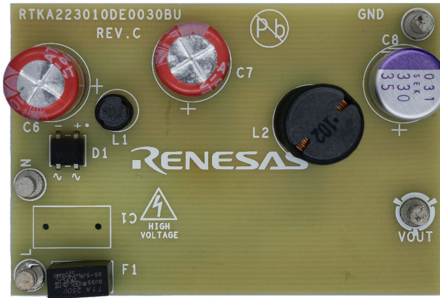
Figure 4. RTKA223010DE0030BU Evaluation Board (Top)
