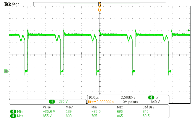
Figure 15. Drain Voltage with 500V AC Input and 21W Short-Time Heavy Load
