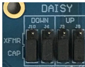
Figure 2. Daisy Jumper Settings
