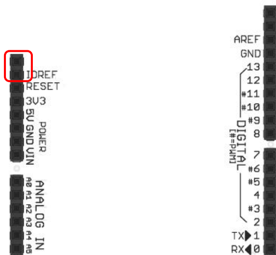
Figure 4-10 : Missing IOREF and Unused Pin on Envision Kit for Arduino™ Rev 3
