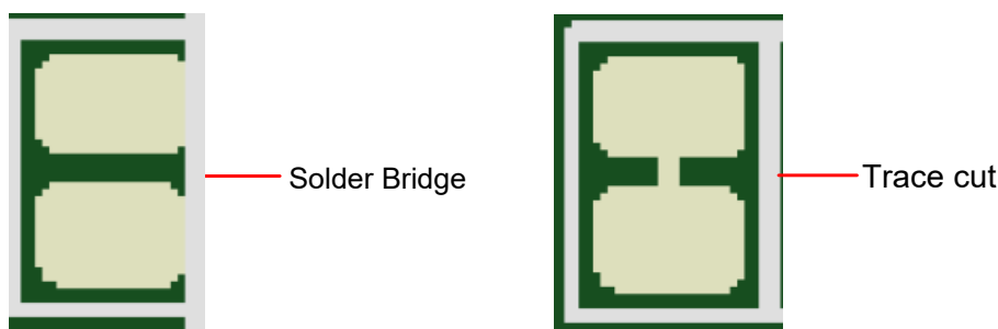
Figure 6-1 Solder Bridge and Trace Cut
