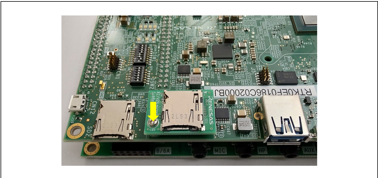
Figure 2.1-4 Use Screw to Fix Sub Board (the photo shows an installed microSD Sub Board)
