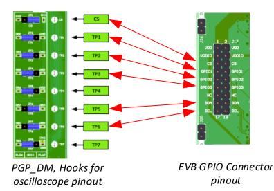
Figure 14. PGP\_DM and SLG51003V-EVB GPIO Connector Pinout Correspondence
