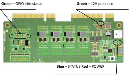
Figure 11. LEDs Location on PGP\_DM
