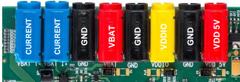
Figure 4: PLT Hardware Power Connections
