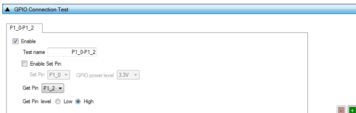
Figure 94: GPIO Connection Tests - DA1468x
