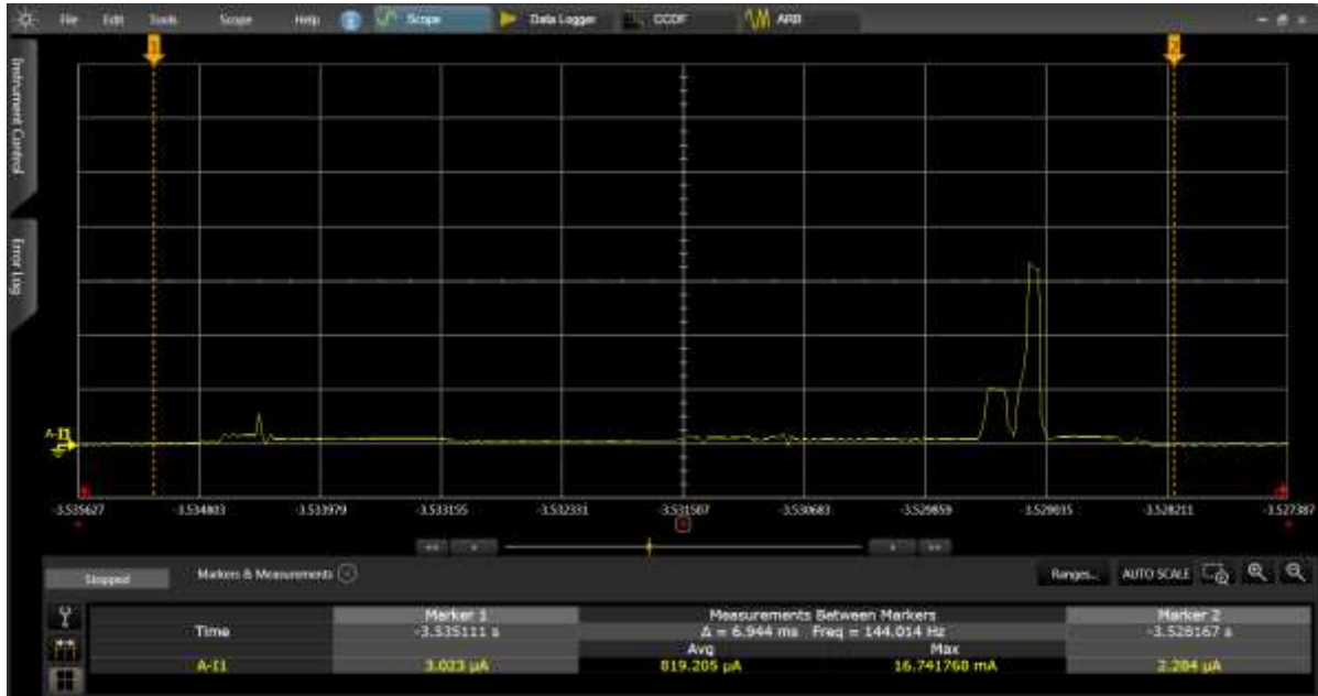
Figure 36: Supply current during a Connection frame
