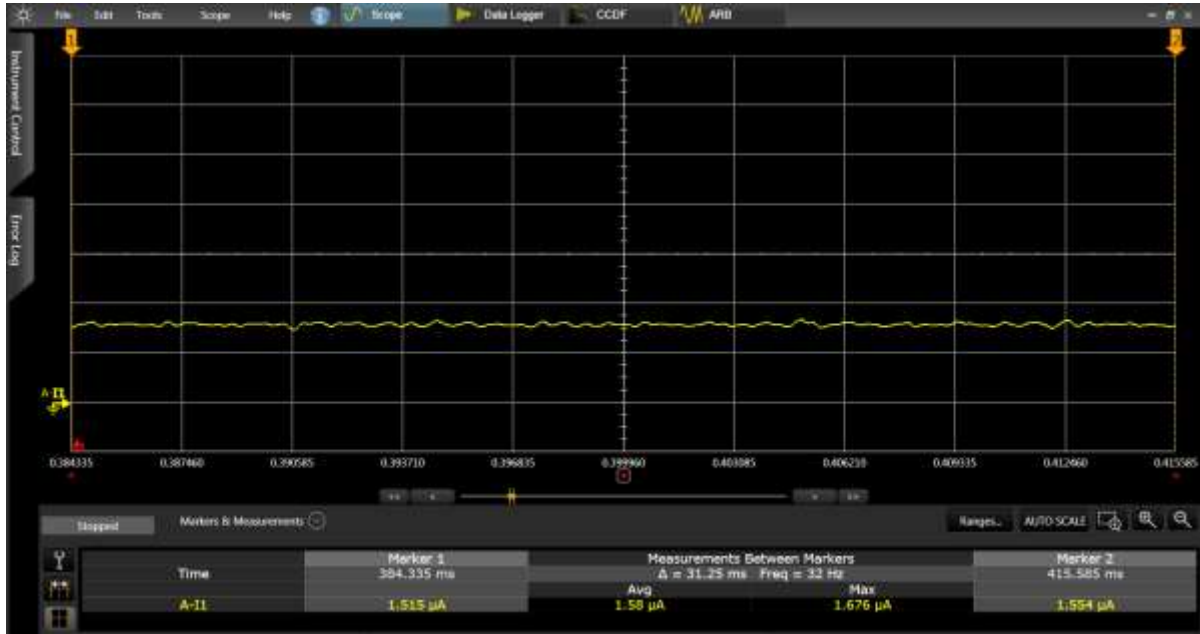
Figure 37: Supply current during Extended Sleep mode
