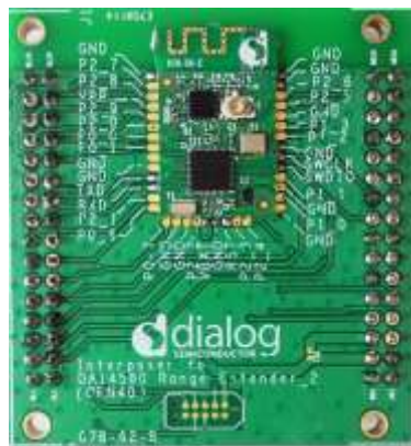
Figure 14: Range Extender v.2 on interposer
