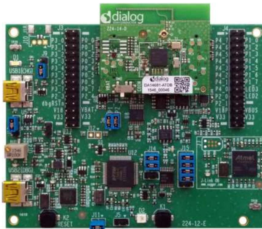
Figure 13: Jumper's placement for Full UART functionality
