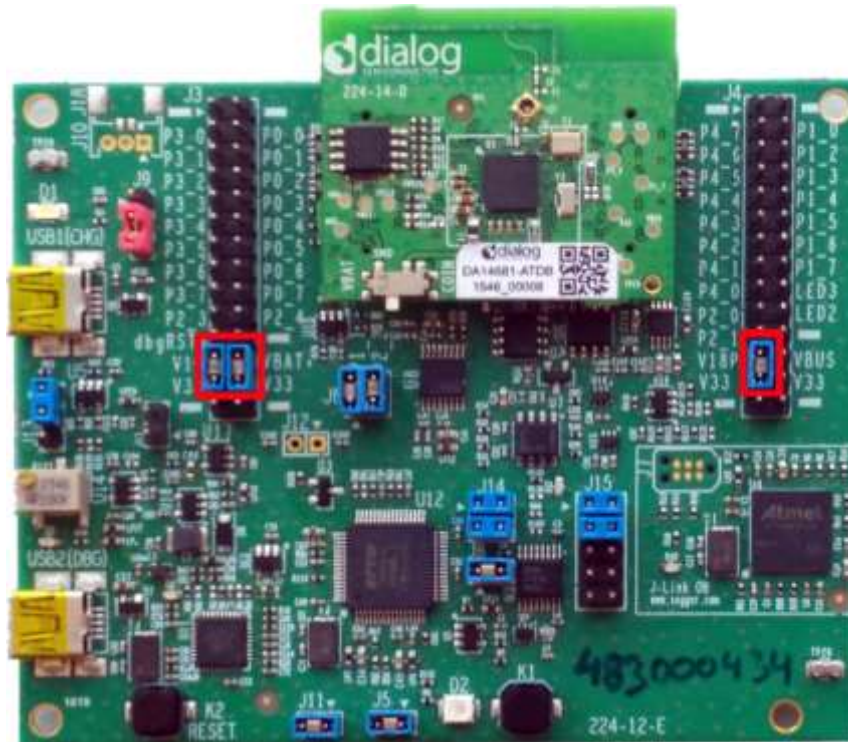
Figure 36 Shorting jumpers for lower VBAT
