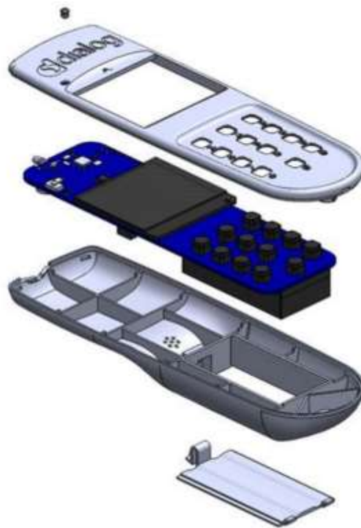
Figure 35: DA14585 Voice RCU Reference Design Enclosure – Top Exploded View
