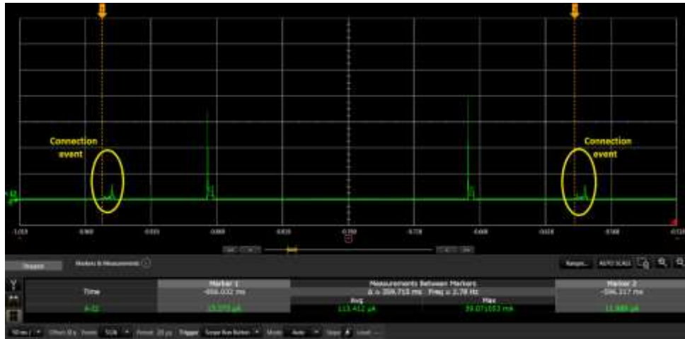
Figure 27: DA14585 Voice RCU Reference Design – Average Operating Current
