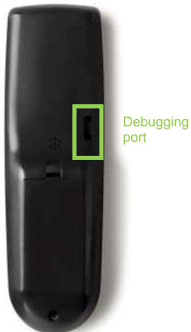
Figure 32: DA14585 Voice RCU Reference Design Enclosure – Bottom View
