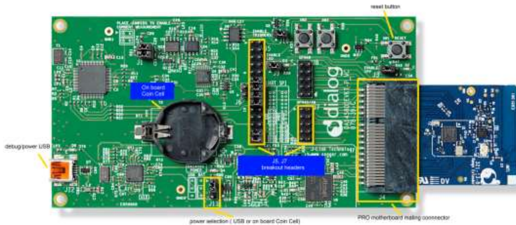
Figure 3: DA14585 Range Extender (321-13-B) on a DA14580 PRO-Dev.Kit Motherboard
