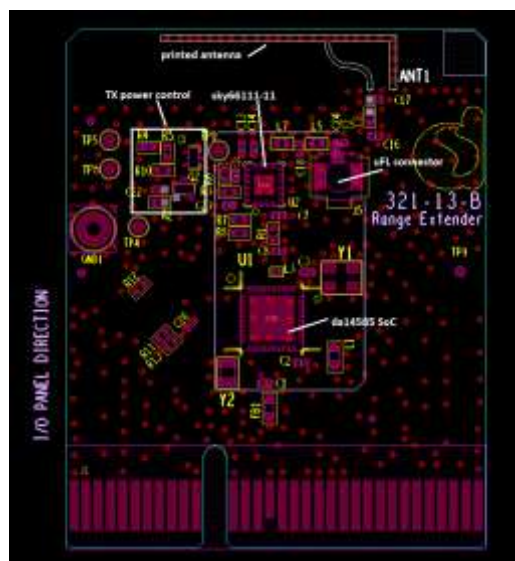
Figure 4: Layout of the DA14585 Range Extender daughterboard
