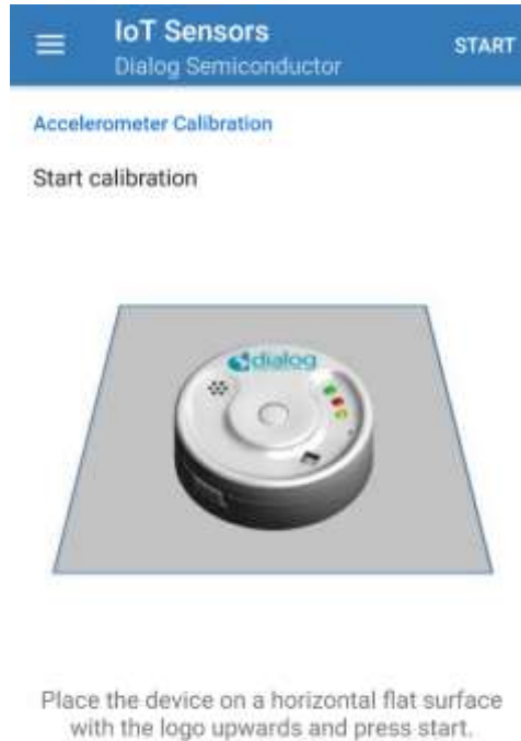
Figure 13: Accelerometer Calibration Settings of Dialog IoT Sensors App
