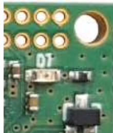
Figure 18: General Purpose Red LED D7
