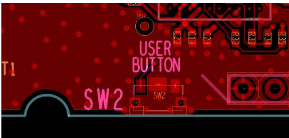
Figure 15: General Purpose Push Button SW2
