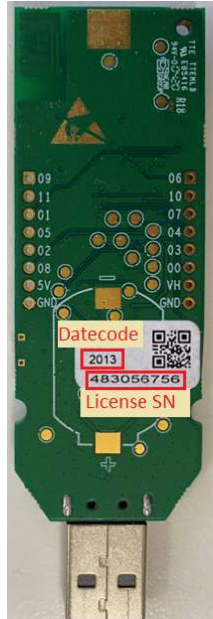
Figure 34: Label on PCBA
