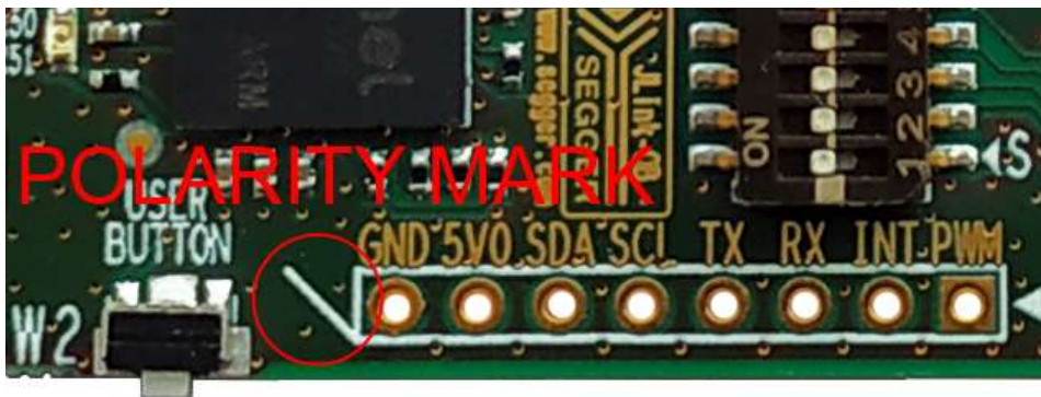
Figure 18: Guides for Proper MikroBus™ Click Board Insertion
