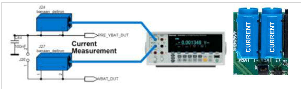
Figure 12: VBAT DUT current measurement setup
