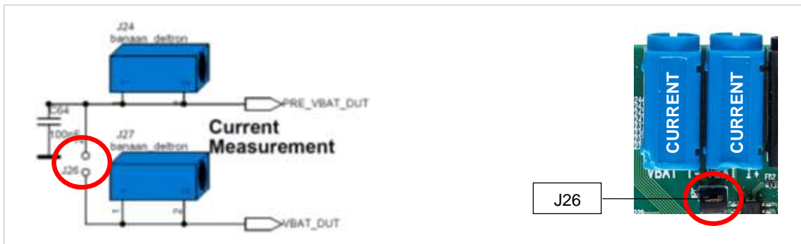
Figure 13: Connections for 'floating current' measurements
