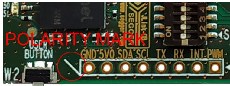
Figure 18. Guides for proper MikroBUS™ click board insertion
