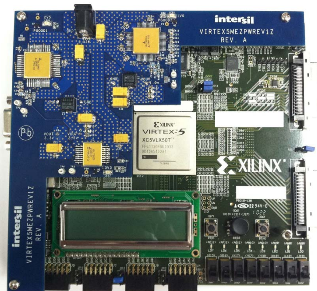
FIGURE 4. RADIATION HARDENED FPGA POWER SOLUTIONS REFERENCE DESIGN
