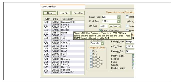
**Note:** EEPROM words  $10_{\text{HEX}}(T_{\text{Config}})$  and  $11_{\text{HEX}}(\text{Osc Trim})$  are trimmed individually during IDT's final test (For more details, see the ZSC31014 Rbic<sub>iLite</sub><sup>TM</sup> Data Sheet). Important: Ensure that these words are not overwritten.
