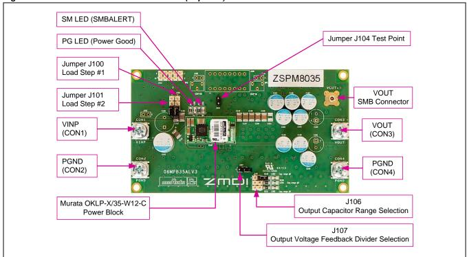
Figure 2.1 ZSPM8035-KIT Evaluation Board (Top Side)
