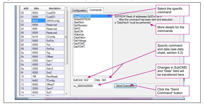
Figure 4.3 Send EEPROM Read Command (Example for Address 02)
