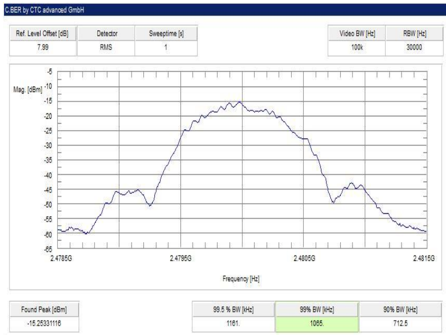
Plot 2: GFSK modulation, highest channel
