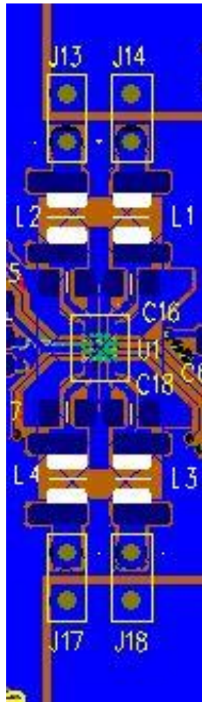
Figure 13: Inductors placement and routing
