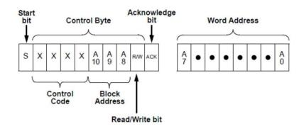
Figure 1. I2C Basic Command Structure
