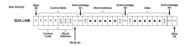
Figure 3. I2C Write Command
