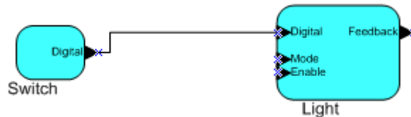
Figure 23 Unicast Network Variable Connection
