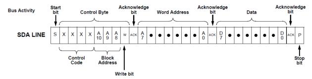
Figure 3. I2C Write Command
