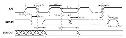
Figure 2. I2C Serial General Timing
