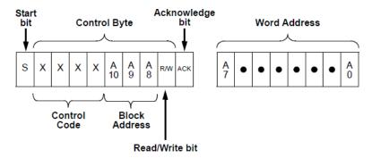
Figure 1. I2C Basic Command Structure
