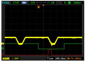
Channel 1 (yellow/top line) – PIN#9 (SDA) Channel 2 (light blue/2nd line) – PIN#8 (SCL)
