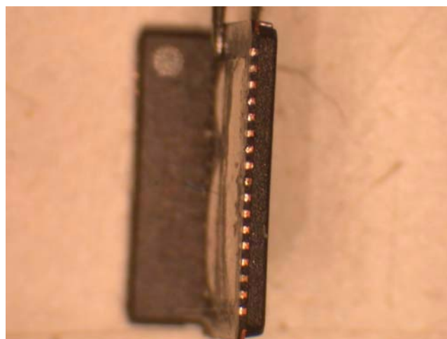
FIGURE 17. FINISHED TINNED THERMAL LAND ON QFN
