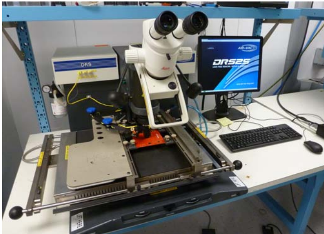
FIGURE 8. REWORK STATION WITH THERMAL PROFILE CONTROL
