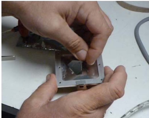
FIGURE 17. DEPOSIT PASTE WITH SMALL SQUEEGEE BLADE
