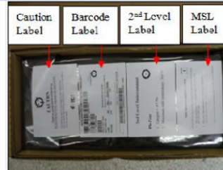
Fig-3 (Paste Inner labels)
