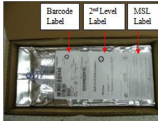
Fig-4 (Paste Inner labels)
