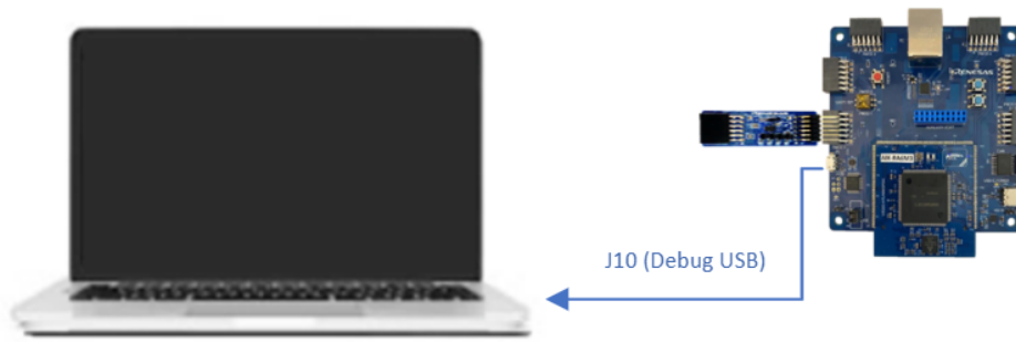
Figure 3. Connecting the AIK-RA6M3 Board to the Host PC via USB Debug Port
