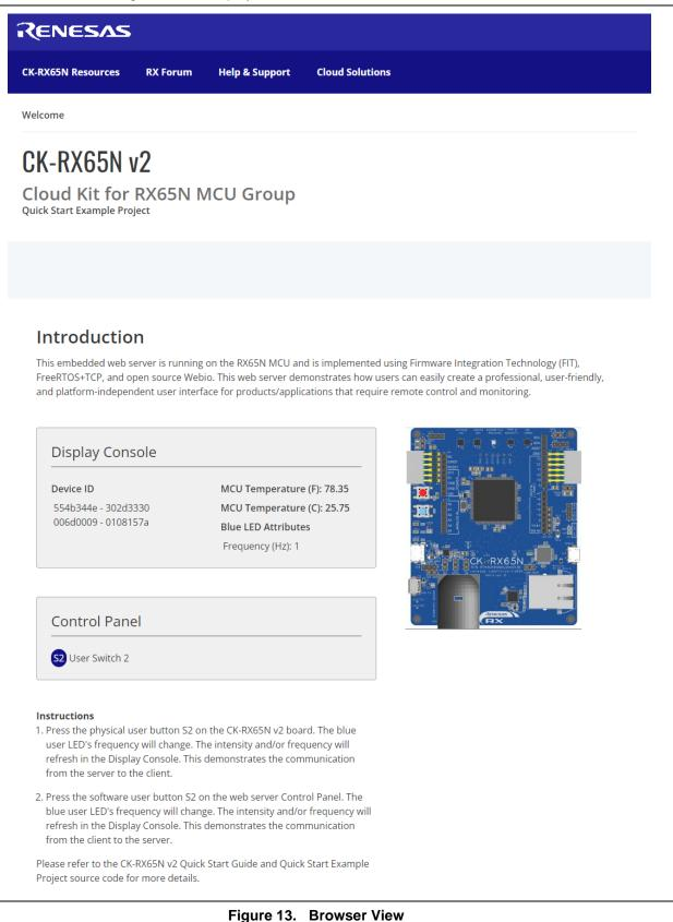
18. Pressing the software user switch S2 on the web page control panel adjusts the flash frequency of the LED4 (blue).
