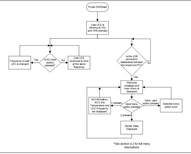
Figure 1. Quick Start Example Project Flow
