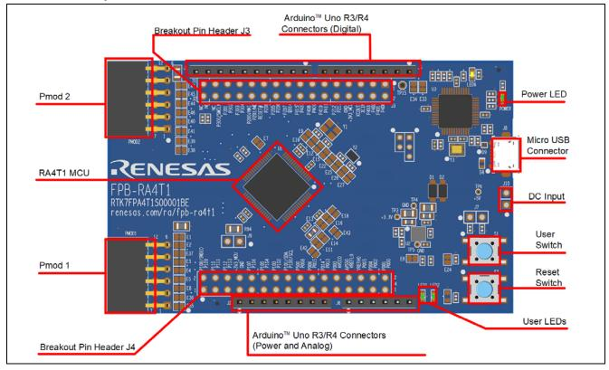
Figure 1. FPB-RA4T1 Board Layout
