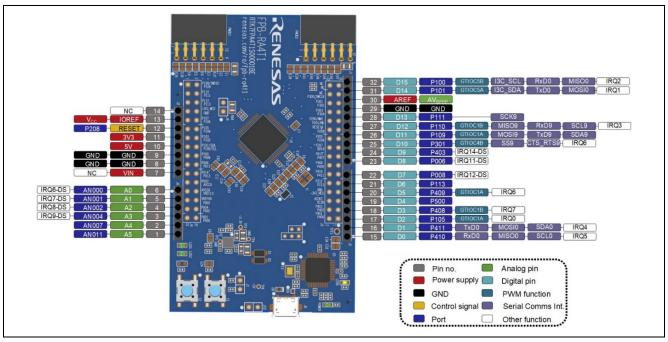
Figure 2. FPB-RA4T1 Arduino Interface
