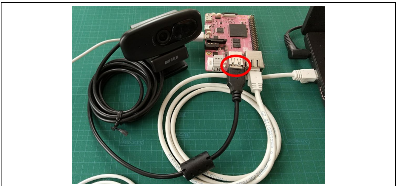
Figure 6-20 Connecting USB camera
