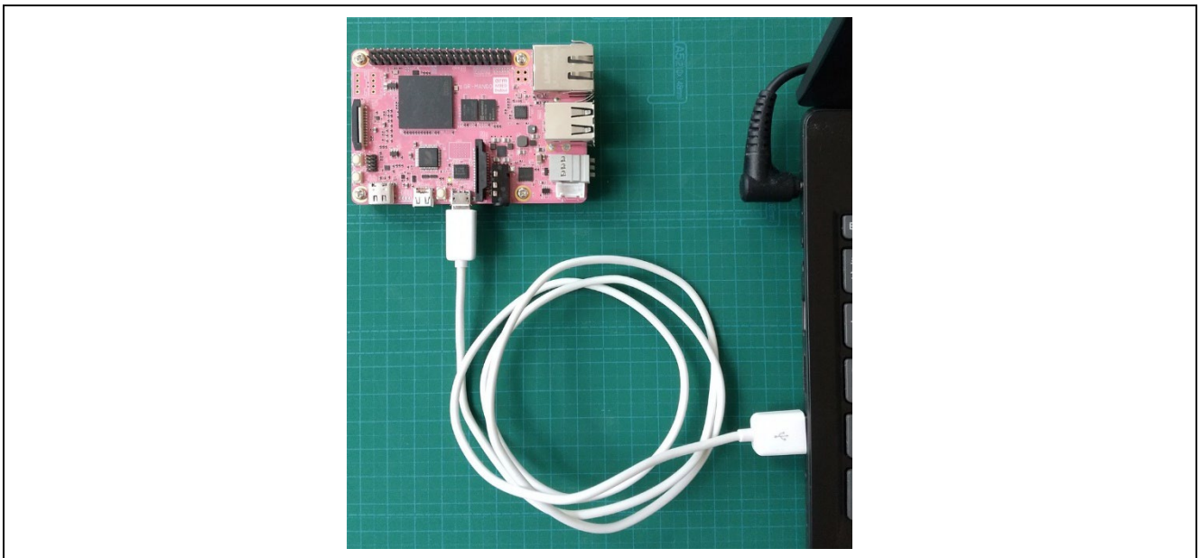
Figure 6-4 Connecting target board and PC
