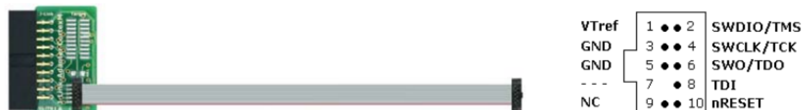
Figure 34. J-Link 9-pin Cortex-M Adapter
