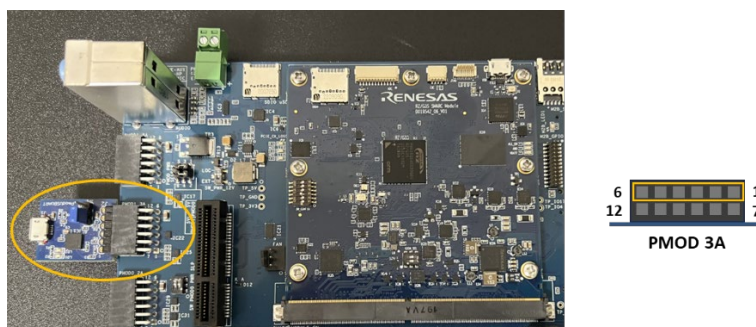
Figure 4-2. Connection between Pmod USBUART and RZ/G3S SMARC EVK
