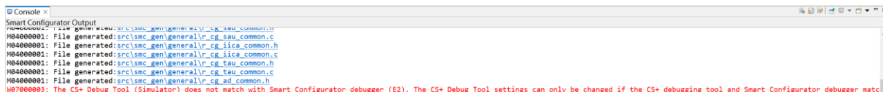
Figure 3-23 The message when CS+ debugging tool/e 2 studio Debug Configurations and Smart Configurator debugger don't match
