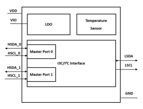
Figure 1. Block Diagram
